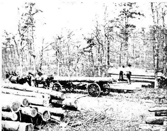
FIG. 55. — A Four-wheeled Log Wagon unloading at a Skidway along a Logging Railroad Spur. The graded right-of-way is being used as a road and, therefore, the logs are being decked from the front of the skidway, instead of from the rear as is the usual custom. Missouri.
